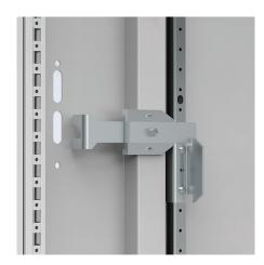
**Description:** Locks or releases the main door after the power has been switched. Universal adapter permits all popular manufacturers variable depth actuators without modification.
