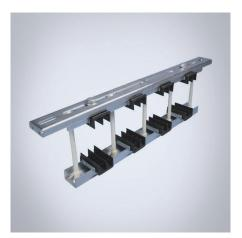
**Description:** Busbar support up to 4500A to be mounted horizontally or vertically. Mounts directly to the enclosure frame or with help of CLPF profiles. Available in one/ two/three bars per phase for bar thickness 10 mm, and width from 30 to 120 mm.
