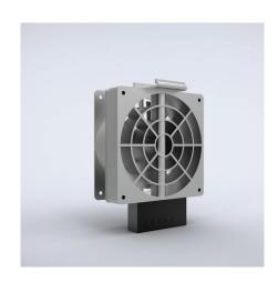
**Description:** High performance space saving fan heater to prevent condensation. The fan assists the natural convection for fast distribution of the heat in large enclosures. Mounting clip for 35 mm DIN rail (EN60715). Temperature safety cutout to protect against overtheating in case of fan failure, automatic reset.
