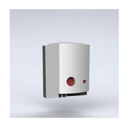
**Description:** High performance heater to prevent condensation. The fan assists the natural convection for a better heat distribution. Double insulated. Mounting clip for 35 mm DIN rail (EN60715). Temperature safety cut-out to protect against overtheating in case of fan failure, automatic reset. Thermostat control lamp.
