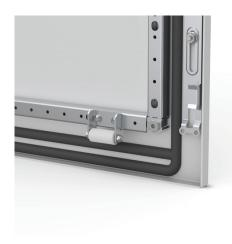
**Description:** For easier closing and positioning of a heavily equipped door (cooling units, etc). Mounted directly to the door frame on the bottom of the door. Highly recommended when fitting loads from 30 kg on the enclosure door.
