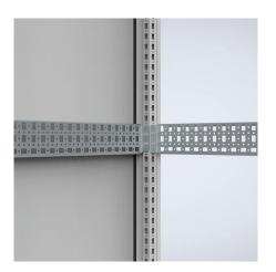
**Description:** Universal profile for both depth and width fitting on the 25 mm DIN hole pattern on the enclosure frame. The 75 mm wide profile is equipped with three rows of holes of which one is turned 90°. This makes it possible to mount the CLPO profiles in both directions. The CLPO increases the useful space by 25 mm.
