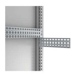
**Description:** Universal profile for both depth and width fitting on the 25 mm DIN hole pattern of the enclosure's frame or in combination with the CLPF and VB profiles. The 75 mm wide profile is equipped with three rows of holes of which one is turned 90°. This makes it possible to mount the CLPF profiles in both directions. The CLPK can be secured by the use of self tapping screws.
