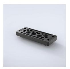
**Description:** Plastic cable entry for a fast, economical and tool-free incoming of cables and/ or pneumatic conduits inside the enclosure. Integrated seal. For snap-in fastening (only for wall thicknesses ranging between 1.4 and 2 mm) and/or screwing. Installation height: 15.5 mm.
