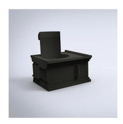
**Description:** Mounted together with the CCF cable gland plate, CCG grommets are used to easily route cables fitted with connectors. The grommet is positioned around the cable and is equipped with catch hooks that anchor themselves in the CCF cable gland plate. Strain relief is achieved by using a simple cable tie.
