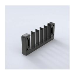
**Description:** Plastic cable entry for a fast, economical and tool-free incoming of cables fitted with connectors, inside the enclosure. Integrated seal. For snap-in fastening (only for wall thicknesses ranging between 1.4 and 2 mm) and/or screwing. Installation height: 14 mm. It has ten openings to be covered with ten CCG cable entry grommets. If it's not necessary to use all the grommets with cables, a dummy grommet is to be used in order to maintain the IP rating.
