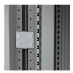
**Description:** Brackets mounted on the outside hole pattern of the frame ensuring a strong and 3 dimensional alignment of the mild steel bayed enclosures with an "auto spacer" function. This method of baying enclosures also has the advantage of creating a direct earthing connection between the enclosure frames.
