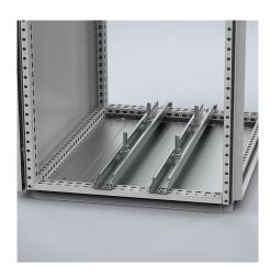
**Description:** Heavy duty carrier bar for mounting heavy components e.g. transformers. Supplied with T-shaped sliding bolts and equipped with slotted holes for mounting in any position, both in width and depth of the enclosure.
