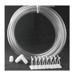
**Description:** Flexible vinyl tube used to direct the cold air for circulation, or to hot spots. Tube connector, end plug, and adhesive clips to hold the tube are included. Holes may be drilled or cut ("V" shaped) in the tube, if the end plug is used at least 6 3.2 mm diameter holes must be made to avoid excessive back pressure on the cooler.
