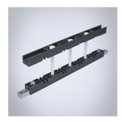
**Beschreibung:** Busbar support up to 1600A to be mounted horizontally or vertically. Mounts directly to the enclosure frame or with help of CLPF profiles. Available in single and double bar per phase for bar thickness 5 mm and only single bar per phase for bar thickness 10 mm, and width from 25 to 80 mm.
