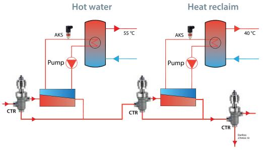
CTR Valve provides Modulating operation to ensure smooth transition avoiding too many Compressor on/off when going from Heat reclaim mode to full through Gas Cooler.
