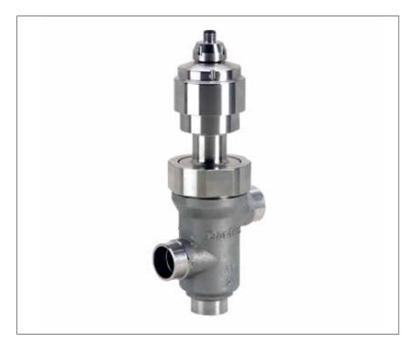
The CTR is an electrically operated 3-way valve designed specifically for operation in  $CO_2$  systems with heat reclaim. CTR is designed to allow full proportional control of the surplus heat from compressor pack into the heat exchanger of transcritical heat reclaim solutions.
