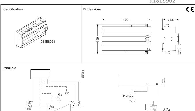
Selection of signal to superheat measurement. Pressure transmitter or temperature sensor S1
