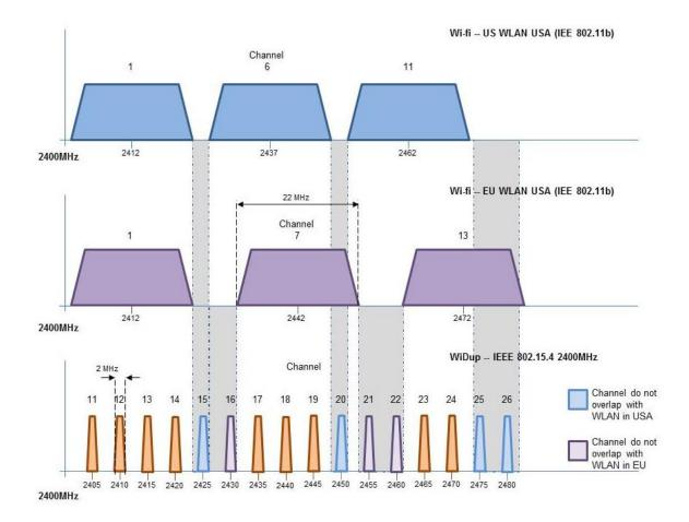
Since channel 15 of WiDup is not overlapping the Wi-Fi bands either in the USA or Europe, it is used by the smart-house system to look for the wireless slave modules present in the field. As for the working band, according to the Wi-Fi channel set in the router, a non-overlapping WiDup channel should be selected: for example, if the router is working on channel 1, channels from 15 to 26 can be selected for the operation of the SH2WBU230N.
