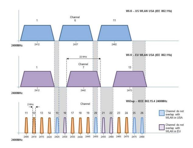
Since channel 15 of WiDup is not overlapping the Wi-Fi bands either in the USA or Europe, it is used by the smart-house system to look for the wireless slave modules present in the field. As for the working band, according to the Wi-Fi channel set in the router, a non-overlapping WiDup channel should be selected: for example, if the router is working on channel 1, channels from 15 to 26 can be selected for the operation of the SH2WBU230N.
