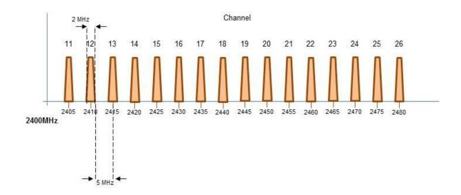
WiDup uses channel 15 to scan the wireless network to find the slave modules and it is fixed, while the working channels can be set from 11 to 26 according to the presence of other systems working at 2.4 GHz.
