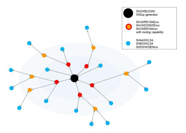
When designing the network, care has to be taken to properly assign the slave modules to the relevant router in order to make them visible to the SH2WBU230N.
