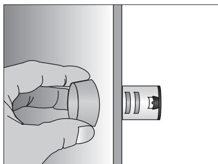
Just insert the pilot light into the hole of the panel.
