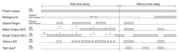
t<sub>v</sub> = Power on delay, t = Time delay (delay on operate and delay on release)
