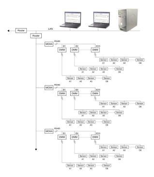
The client (or clients) is also connected to the LAN. The client is the application for the operator of the system, who wants to receive information from the parking facility. The design of the parking facility is done by means of the client, where diagrams, pictures etc. can be uploaded as background for the programming.
