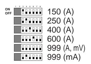
3, 4, 5, 6, 7 and 8 according to what is shown in the figure on the left. The different position of the decimal point allows you to change these scales into either: **15.0** -**25.0** - **40.0** - **60.0** - **99.9** or **1.50** - **2.50** - **4.00** - **6.00** - **9.99**. Direct connection: set the dipswitches for 1A measurement as per 999 (mA).
