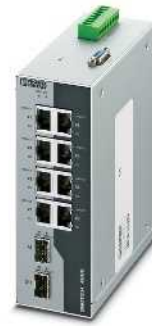
8 ports RJ45 et 2 ports SFP
