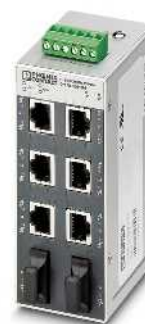
6 ports RJ45 et 2 ports FO (monomode)
