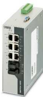
6 ports RJ45 et 2 ports FO (multimode)
