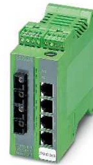
4 ports RJ45 et 2 ports FO (multimode)
