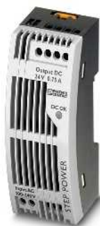
Alimentation, 1 AC, 24 V DC, 0,75 A, Type plat
