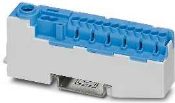
16 (25) mm 2 , 80 A, bornier, 15 raccords
