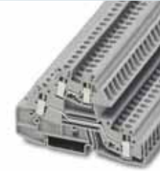
4 (4) mm 2 , 32 A, three-level terminal block, 1 x L phase conductor, 2 x L phase conductor
