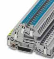
4 (4) mm 2 , 32 A, three-level terminal block, 1 x L phase conductor, 1 x N conductor, 1 x PE
