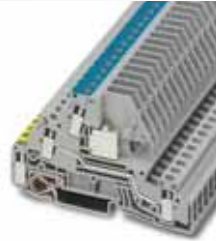
4 (4) mm 2 , 32 A, three-level terminal block, 1 x L phase conductor, 1 x N conductor can be disconnected, 1 x PE
