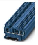
Feed-through terminal block, without actuation lever, Connection method: Push-in connection, Cross section: 0.14 mm<sup>2</sup> - 4 mm<sup>2</sup>, AWG: 26 - 12, Width: 5.2 mm, Height: 35.2 mm, Color: blue, Mounting type: NS 35/7,5, NS 35/15
