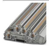
Installation level terminal block, Push-in connection, Cross section: 0.2 mm<sup>2</sup> - 6 mm<sup>2</sup>, AWG: 24 - 10, Width: 6.2 mm, Color: gray, Mounting type: NS 35/7,5, NS 35/15
