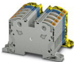
High-current terminal block, Connection method: Power-Turn connection, Cross section: 2.5 mm 2 - 35 mm 2 , AWG: 12 - 2, Width: 64 mm, Height: 68.3 mm, Color: gray/black-yellow, Mounting type: NS 35/15
