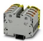
High-current terminal block, Connection method: Power-Turn connection, Cross section: 2.5 mm² - 35 mm², AWG: 12 - 2, Width: 64 mm, Color: gray/black-yellow, Mounting type: NS 35/15
