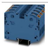
High-current terminal block, Connection method: Power-Turn connection, Cross section: 2.5 mm<sup>2</sup> - 35 mm<sup>2</sup>, AWG: 12 - 2, Width: 16 mm, Color: blue, Mounting type: NS 35/15
