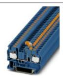
Knife disconnect terminal block, Connection type: Push-in connection, Cross section: 0.2 mm² - 6 mm², AWG: 24 - 10, Nominal current: 20 A, Nominal voltage: 400 V, Length: 56 mm, Width: 6.2 mm, Color: blue, Assembly: NS 35/7,5, NS 35/15
