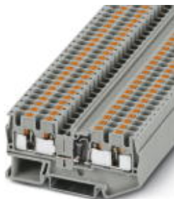
Component terminal block, with integrated diode, Connection method: Push-in connection, Cross section: 0.2 mm 2 - 6 mm 2 , AWG: 24 - 10, Width: 6.2 mm, Color: gray, Mounting type: NS 35/7,5, NS 35/15
