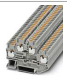
Component terminal block, for installing components that can be individually selected, Cross section: 0.14 mm² - 4 mm², AWG: 26 - 12, Connection type: Push-in connection, Width: 5.2 mm, Color: gray, Mounting type: NS 35/7,5, NS 35/15
