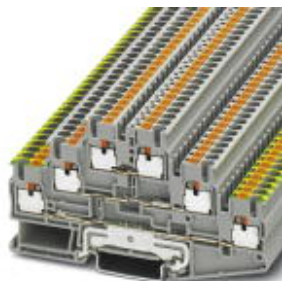
Ground modular terminal block, Connection method: Push-in connection, Cross section: 0.14 mm 2 - 4 mm 2 , AWG: 26 - 12, Width: 5.2 mm, Color: gray/green-yellow, Mounting type: NS 35/7,5, NS 35/15
