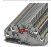
Disconnect terminal block, double level with angled contour and two disconnect points, Connection type: Push-in connection, Cross section: 0.14 mm² - 4 mm², AWG: 26 - 12, Nominal current: 20 A, Nominal voltage: 400 V, Length: 127.5 mm, Width: 5.2 mm, Color: blue, Assembly: NS 35/7,5, NS 35/15
