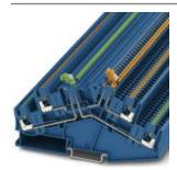
Knife disconnect terminal block, Double level with angled contour and two disconnect knives, Connection type: Push-in connection, Cross section: 0.14 mm² - 4 mm², AWG: 26 - 12, Nominal current: 16 A, Nominal voltage: 400 V, Length: 127.5 mm, Width: 5.2 mm, Color: blue, Assembly: NS 35/7,5, NS 35/15
