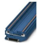
Knife disconnect terminal block, same shape as disconnect terminal block, Connection type: Push-in connection, Cross section: 0.14 mm<sup>2</sup> - 1.5 mm<sup>2</sup>, AWG: 26 - 14, Nominal current: 17.5 A, Nominal voltage: 400 V, Length: 58.9 mm, Width: 3.5 mm, Color: blue, Assembly: NS 35/7,5, NS 35/15
