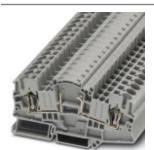
Component terminal block, for installing components that can be individually selected, Connection method: Spring-cage connection, Cross section: 0.2 mm² -10 mm², AWG: 24 - 10, Width: 8.2 mm, Color: gray
