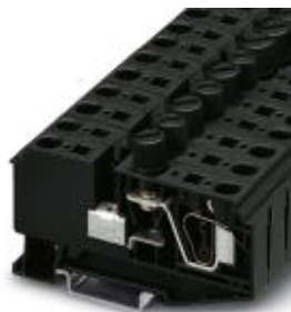
Spring-cage fuse terminal block for cartridge fuse inserts with indicating pin screw cap, cross section: 0.5 - 6 mm², width: 12 mm, color: black
