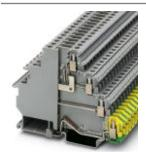
Installation ground terminal block, Cross section: 0.2 mm² - 4 mm², AWG: 24 - 12, Connection type: Screw connection, Width: 6.2 mm, Color: gray, Mounting type: NS 35/7,5, NS 35/15
