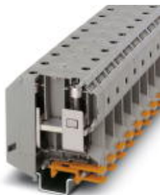
High-current terminal block, Connection method: Screw connection, Cross section: 25 mm 2 - 95 mm 2 , AWG: 4 - 3/0, Width: 25 mm, Height: 90 mm, Color: gray, Mounting type: NS 35/15, NS 32
