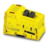
Safety-oriented decentral relay output module, IP20 degree of protection, for the INTERBUS-Safety and the PROFIsafe system. This module has four safe digital relay outputs, each having two contacts.
