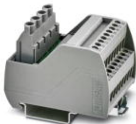
VARIOFACE module, with two equipotential busbars (P1, P2) for potential distribution, for mounting on NS 35 rails. Module width: 131.5 mm
