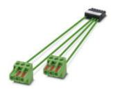
Cable set for signal transmission on the termination carrier for safety relay modules from the PSR-FSP series. Connection of terminal points A1 and A2 (signal transmission) as well as 31 and 32 (confirmation contact) with screw connection to the signal PCB via a 6-pos. PTSM connector.
