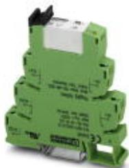
PLC-INTERFACE, consisting of PLC-BPT.../21-21 basic terminal block with push-in connection and plug-in miniature relay with multi-layer gold contact, for mounting on DIN rail NS 35/7,5, 2 PDTs, input voltage 230 V AC/DC
