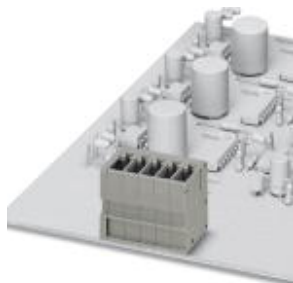
ST-COMBI receptacle, plug-in direction vertical to the PCB, pitch: 5.2 mm, no. of positions: 11
