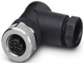
Connector, 5-position, Socket angled M12, A-coded, Screw connection, Knurl material: Zinc die-cast, nickel-plated, Cable gland Pg9, External cable diameter 6 mm ... 8 mm
