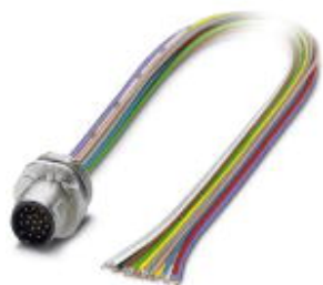
Sensor/actuator flush-type plug, 17-pos., M12 SPEEDCON, front/screw mounting with M16 thread, with 0.5 m PVC litz wire, 17 x 0.14 mm 2
