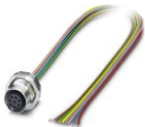
Sensor/Actuator flush-type socket, 8-pos., M12, A-coded, rear/screw mounting with Pg9 thread, with 0.5 m TPE litz wire, 8 x 0.25 mm 2 , on high-grade steel version
